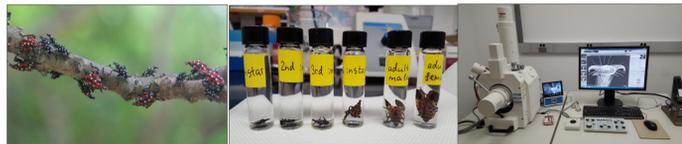
Tissue fixation was done using modified hexamethyldisilazane drying technique. The morphology of the stylets and tarsal tips were investigated, size measurements were taken (Fig. 1), and all the morphological structures were photographed.
